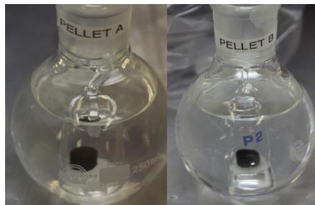
Fig. 7. Pellet A, left and pellet B, right, in their leaching flasks.
